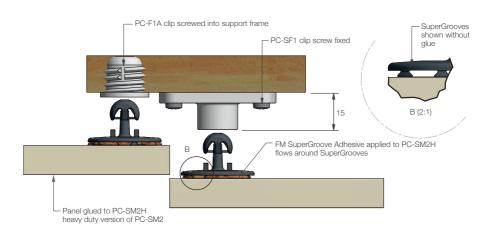
The Fastmount® multi-award winning system has revolutionized the mounting of panels. Panels can easily be removed and refitted in any sequence time after time. For further information or technical support contact: info@fastmount.com
